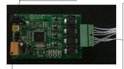
B.S-BUS connection (DC24+, D+, D-, GND)
